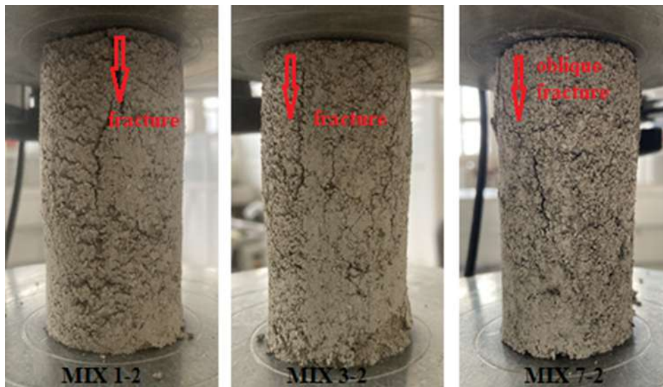
Figure 7. After F-T fracture patterns
